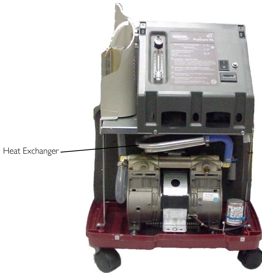
FIGURE 6.8 Cleaning the Heat Exchanger
